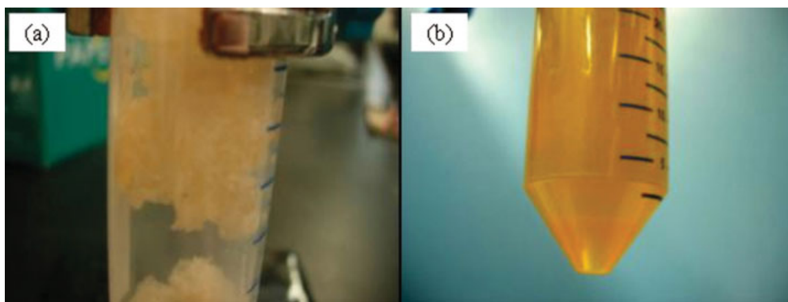
Figure 2 Photos showing 18 wt % CS solutions: (a) prepared by the conventional method (direct dissolution) and (b) prepared by the new method (dilute dissolution and evaporation-concentrating). [Color figure can be viewed in the online issue, which is available at www.interscience.wiley.com .]
